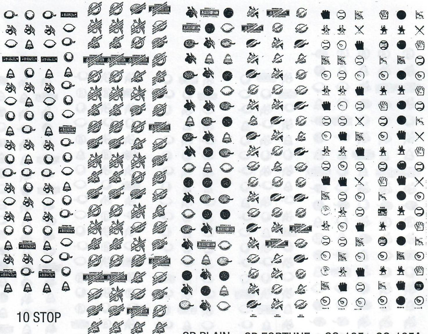
The first and second set of reel strips on this page are used on Mills Machines of the 1920-1940 era. The ten stops, used on all Goosenecks and early Escalator Machines. The third and fourth set are the SP's which were used on Mills Machines of the thirties. The fifth set, CC-135 was used on the baseball vendors of the 1920's. The last set on this page was used on the Mills Baseball Machine with the free play feature.
